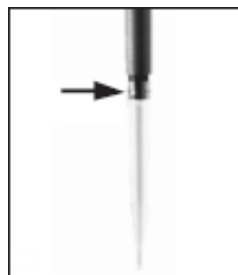
Fig. 3: Attaching the Pipette Tips
